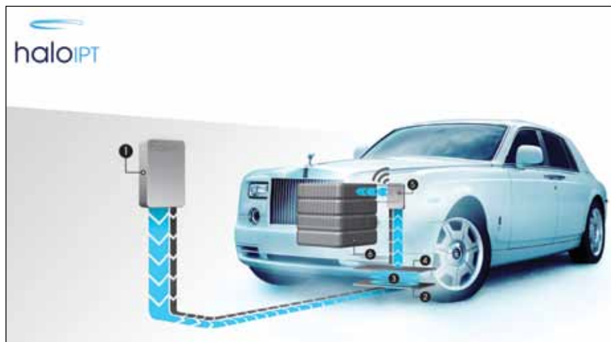
1 POWER SUPPLY 2 TRANSMITTER PAD 3 WIRELESS ELECTRICITY & DATA TRANSFER 4 RECEIVER PAD 5 SYSTEM CONTROLLER 6 BATTERY
